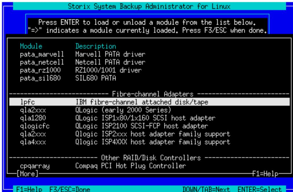
After loading the module for the HBA, **only the underlying paths are listed and no dm-multipath devices were created**. At this point it is necessary to also load the device handler for the SAN.
